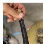
Check the condition of the hose, its use-by date and the seal. Screw the end of the hose into the new bottle (don't forget the seal).
